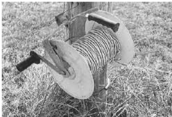
Figure 5. Geared reels for polytape or polywire allow easy installation of temporary electric fences in paddocks.
