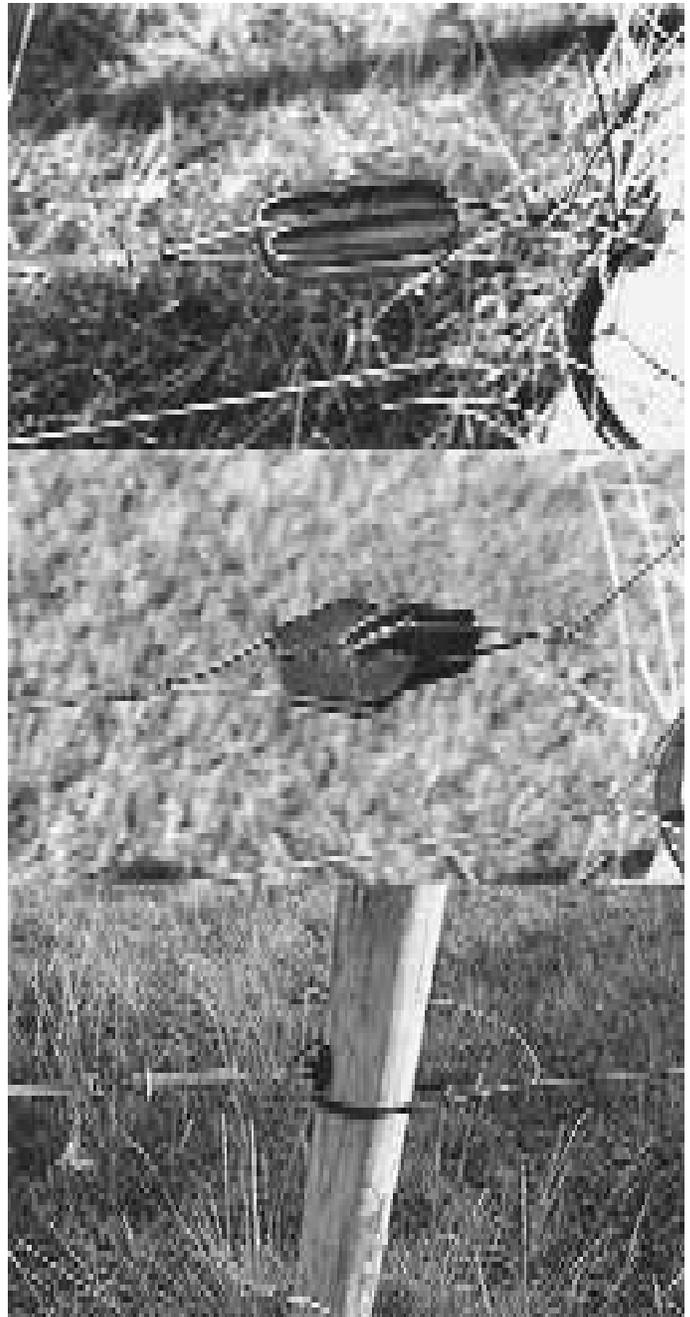
Figure 7. Three types of insulators for corners and ends of high-tensile wire fences. (Top) Ceramic. (Middle) Polyethylene or polypropylene. (Bottom) Wrap-around tube-type insulator.
